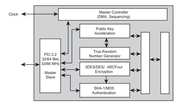
The **BCM5821** Super E-commerce Processor is a high-performance public-key processor, able to perform over 4000 SSL/TLS sessions per second and 3000 IKE negotiations per second. The high level of performance and integration in the **BCM5821** makes it ideal for high-performance embedded applications with footprint and power limitations.
